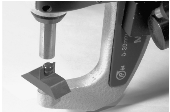
Fig. 10. Arrangement to determine the notch length (ligament thickness). The thickness of the measuring blade is adjusted to the notch width. The tip of the blade is sharpened, so that the blade can reach the notch root even if the corners of the notch are rounded. The measurement aid is positioned between the callipers of the micrometer screw. Measured is the difference between the edge of the blade and the top position of the ball.
